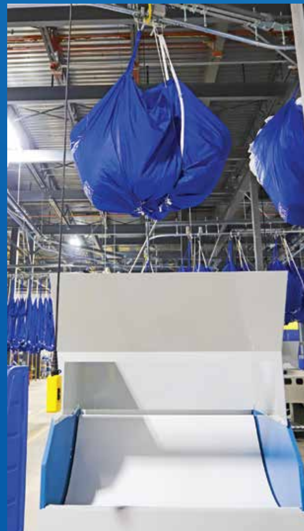
Automatically lift and move linen towards the folding operator
