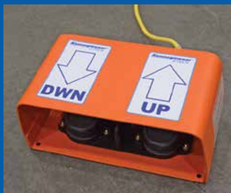
controlled by the operator through the foot pedal
