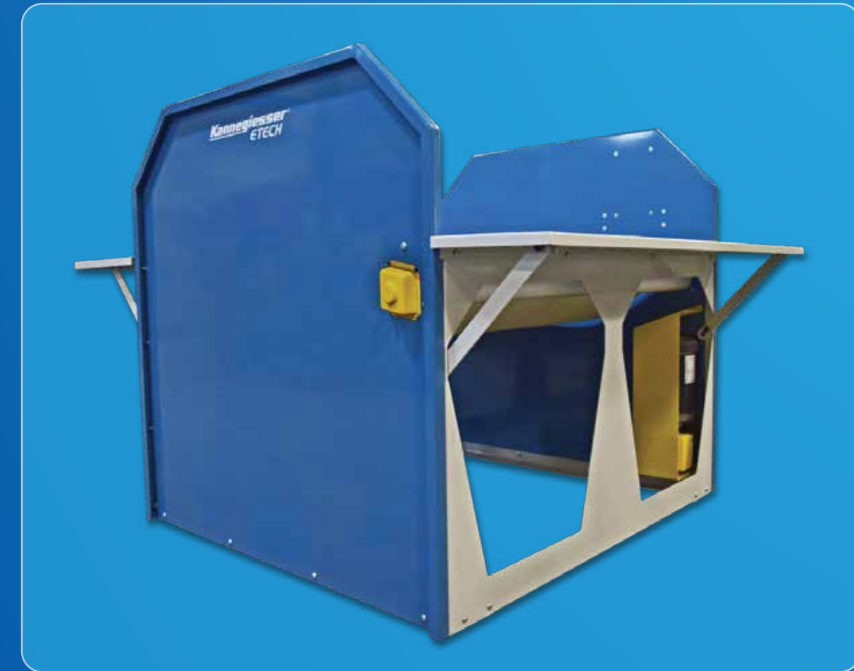
Automatically lift and move linen towards the folding operator
