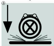
• Then slide on the coupling and align with the marks on the pipe ends. Slightly tighten the screws alternately using a ratchet or screwdriver. Stop turning the coupling once the coupling teeth are in engagement with the pipe. Use a dynamometric key to alternately tighten the screws.
