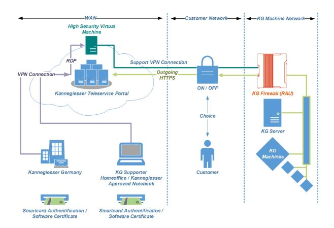
The Kannegiesser teleservice portal ("WAN" section) forms the central unit of the remote maintenance concept and is a closed communication environment. This portal is physically located in a high availability cloud with backup scenarios, uninterruptible power supply and fastest internet connections.
