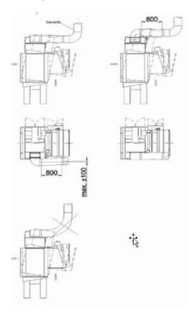
Exhaust air connection upwards
