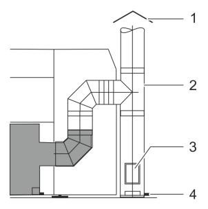
The bright section of the exhaust gas guide is to be installed by the ironer owner/user. Guidance must comply with the local, valid regulations. Contact the local, responsible authorities.
